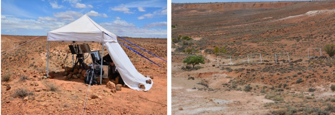
Figure 2. Measurement set-up from a conducted campaign. Sensor for continuous image recording (left) and hot arid scene with mounted scaffolds for fixation of camouflage nets (right).
