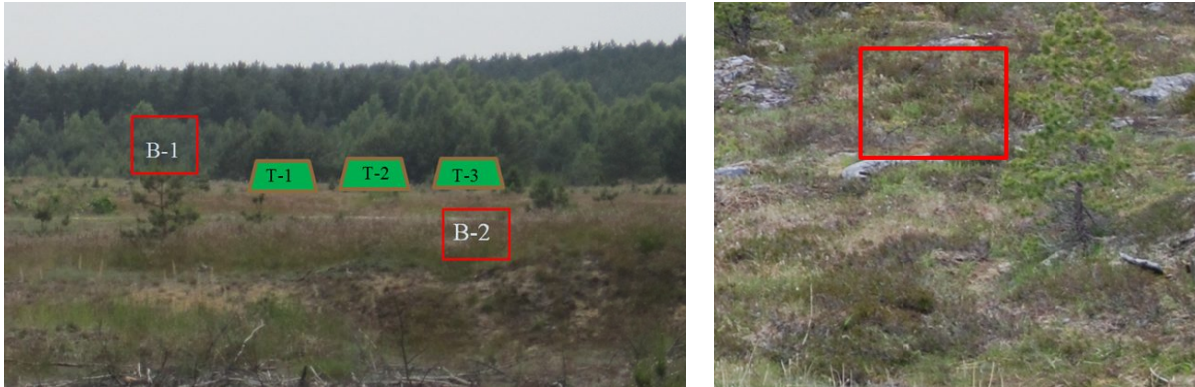
Figure 3. Example of woodland background elements containing forest line (B-1) and heather (B-2) in a scene along with the nets (indicated with T's) that are under evaluation. Note that B-2 in a realistic test should be moved closer to the net garages to ensure equal distances to the sensor. The right image shows a close-up image of heather.
