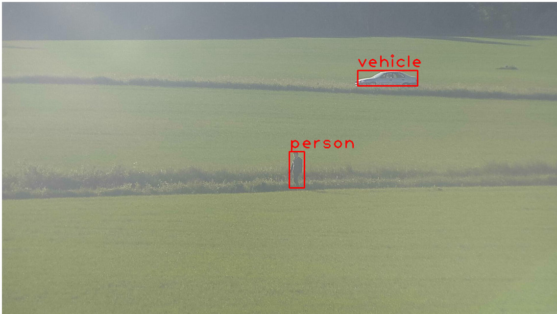
Figure 2.7 DNN detector run at range on a typical high resolution image from the PTZ camera.
