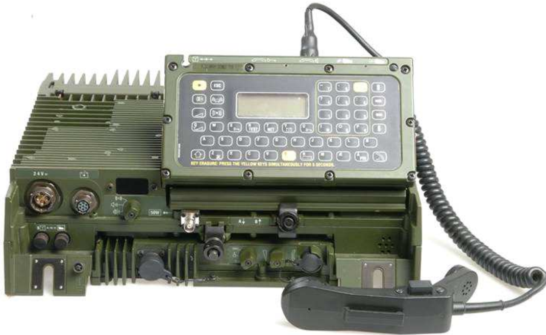
Figure 2.14 The Kongsberg vehicle mounted MRR, from publicly available data sheet [8].
