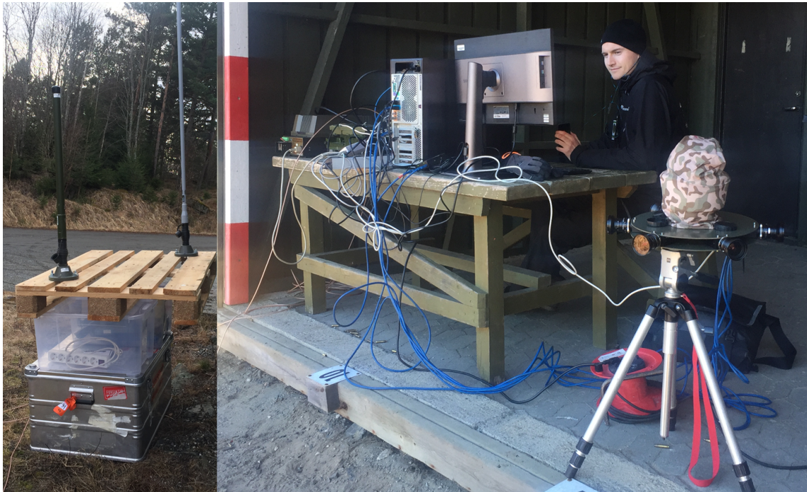
Figure 4.2 The UGS sensor setup with the UHF and VHF antennas on the left.
