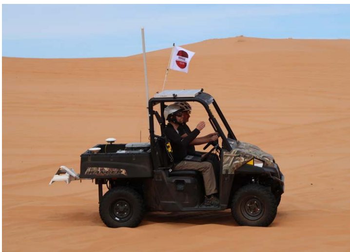
◀ RIMFAX Instrument mounted on an electric vehicle simulating the Mars rover in Utah in 2018. The image above: RIMFAX sounding from Coral Pink Sand Dunes in Utah showing subsurface sedimentary layers.
