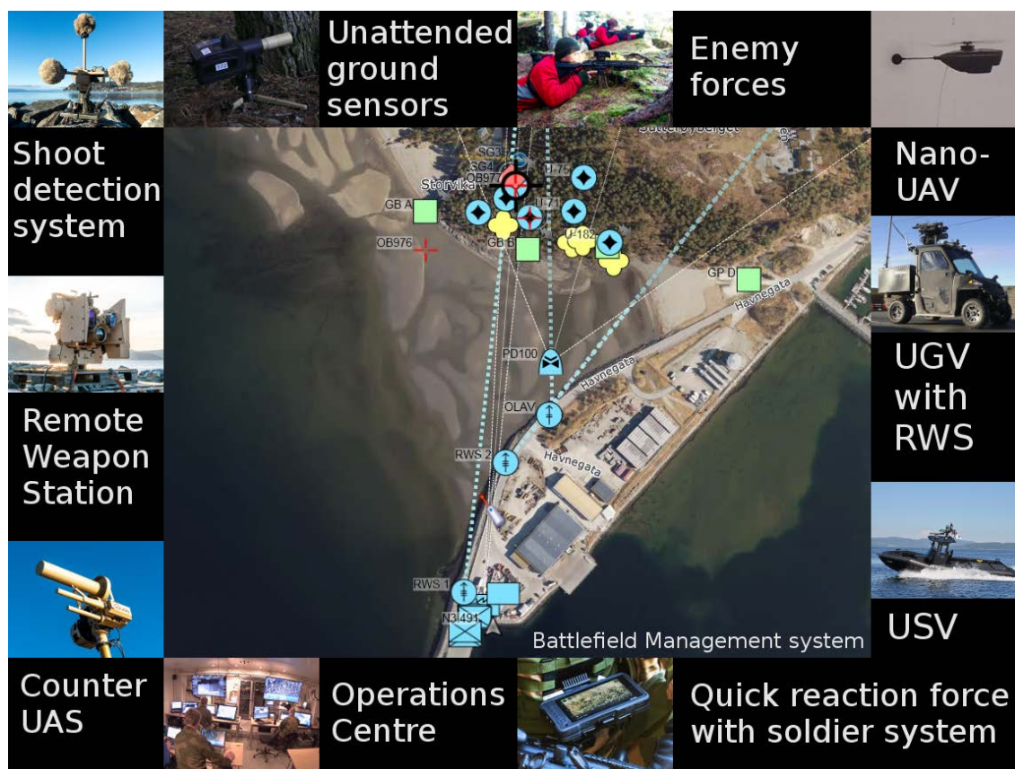
Figure 3.1 All main components of the base defence system are shown along the figure border. The map in the centre shows the positions of all sensors and effectors. RWS1 and RWS2 are two stationary remote weapon stations, OLAV is a UGV with a remote weapon station, PD100 is a nano-UAV, and Odin is a USV patrolling the sea side (not shown in the map). The control centre is to the south of the map, and the unattended ground sensors are to the north.
