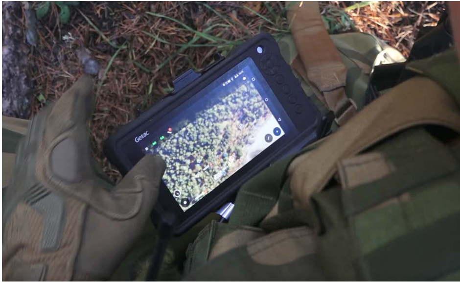
Figure 4.7 Soldier C2 system, PDA mounted to soldiers' load carrying vest.
