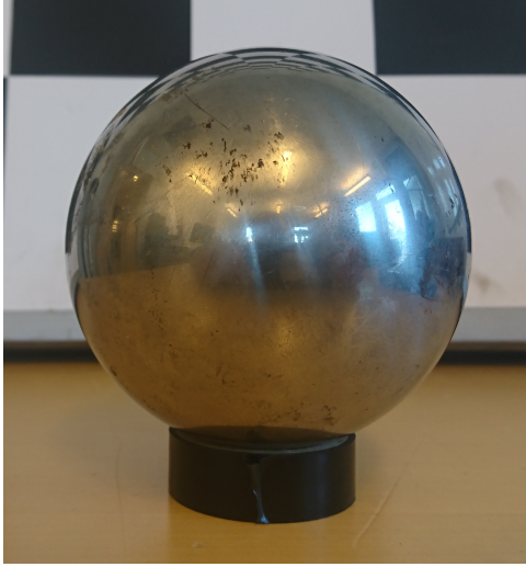
(a) 100mm diameter solid stainless steel ball bearing sphere
