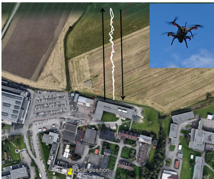
(a) Experimental setup of UAV flying outwards, turning, and flying inwards
