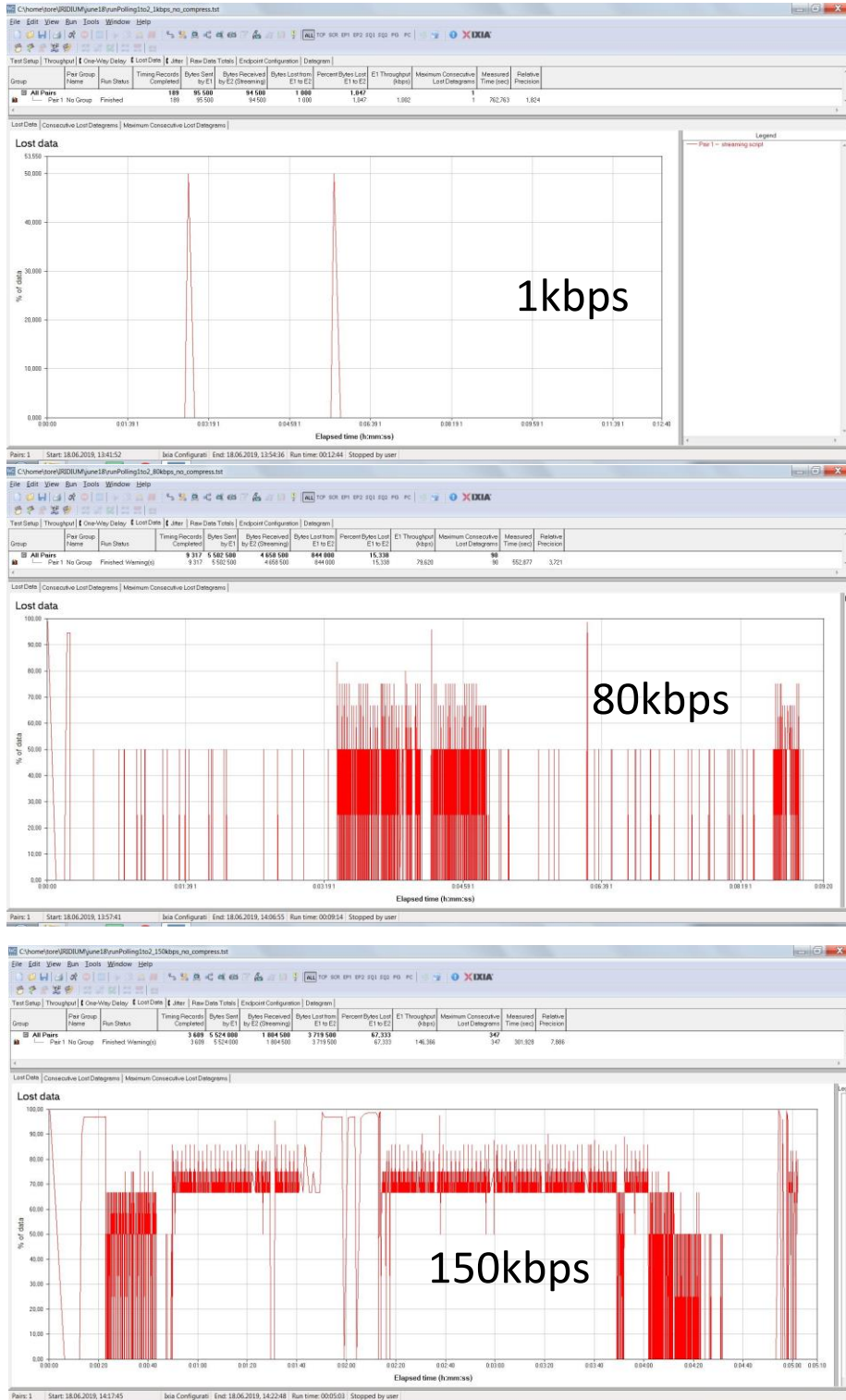
Figure 4.4 Measured loss at constant load {1, 80, 150} kbps.
