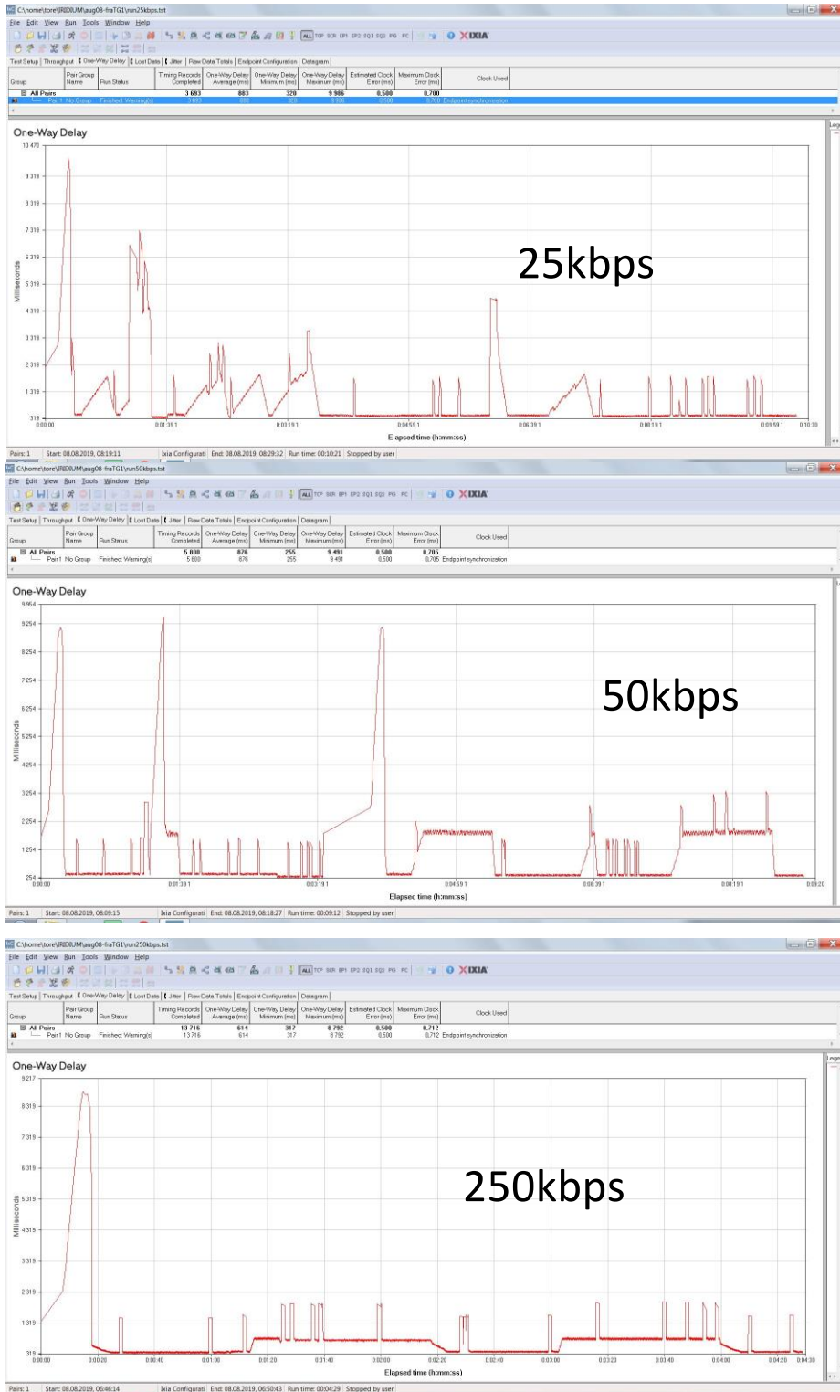
Figure 5.3 Measured delay at constant load {25, 50, 250} kbps.
