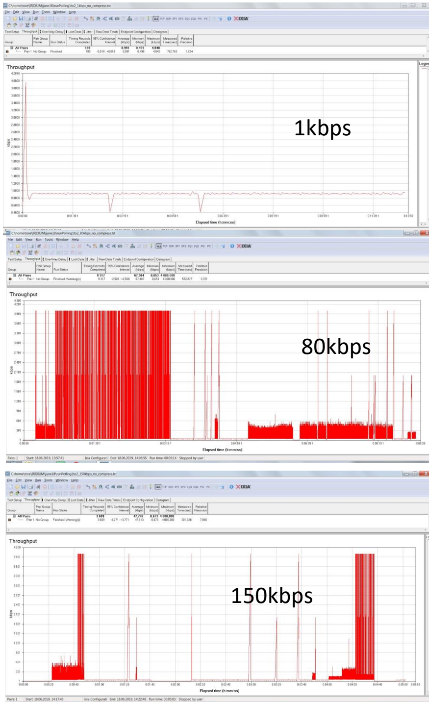
Figure 4.3 Measured throughput at constant load {1, 80, 150} kbps.
