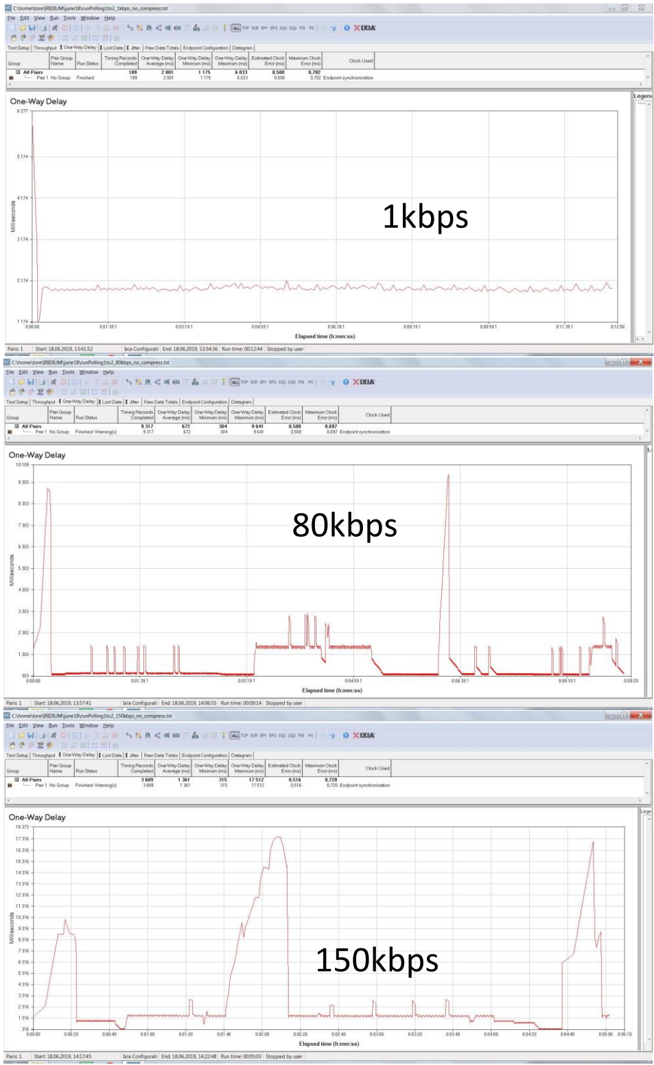
Figure 4.5 Measured delay at constant load {1, 80, 150} kbps.
