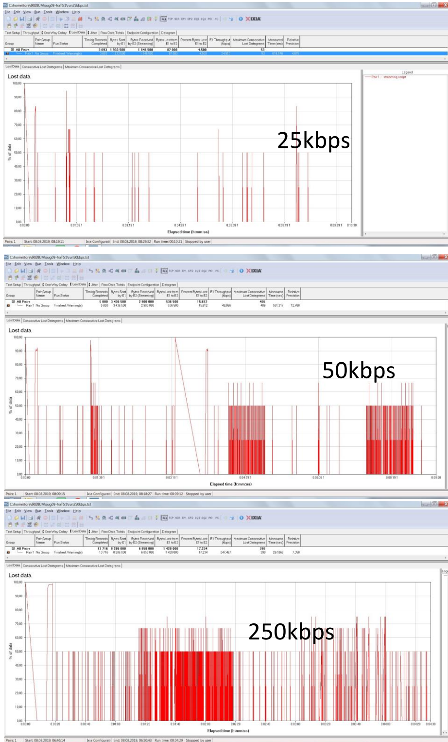
Figure 5.2 Measured loss at constant load {25, 50, 250} kbps.
