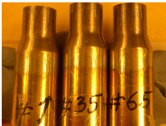
Figure 8.1 Used casings with circular impressions of the conformal sensor. Shot numbers are visible.
