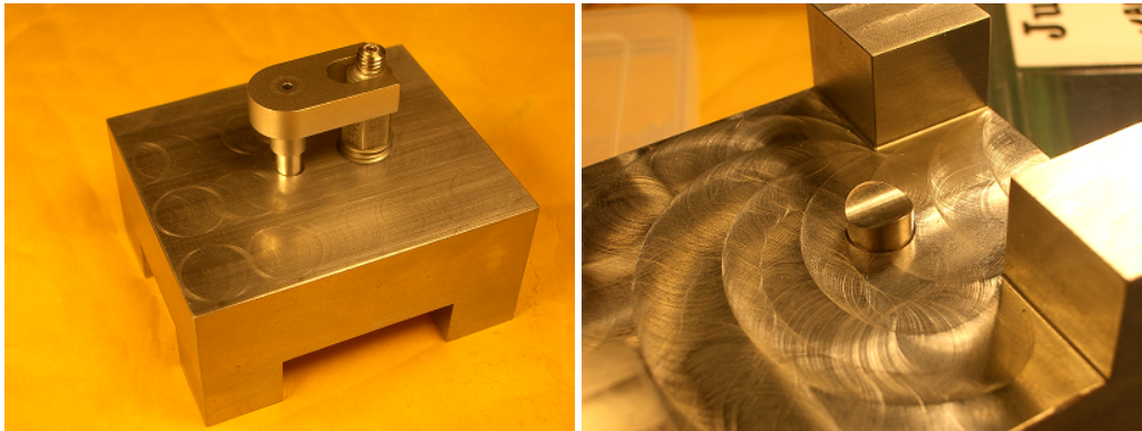
Figure 7.6 Device for measuring sensor seating depth change, top and bottom view.
