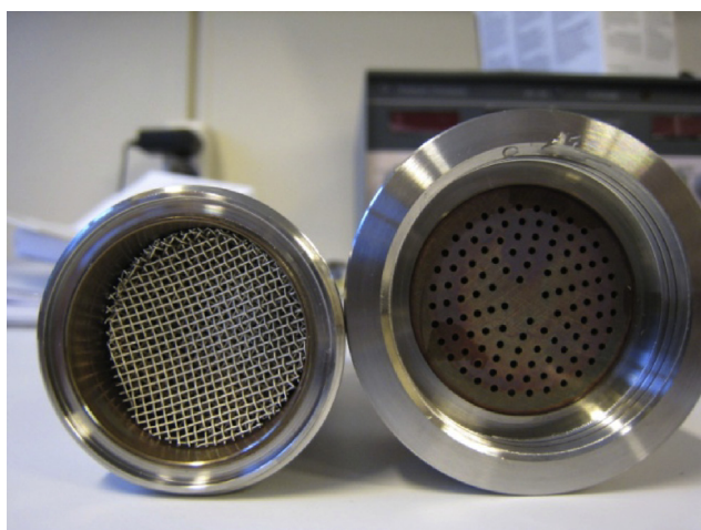
Fig. 4 – Top internal view of the reactor (left) with top end cap (right). The reactor is filled with a silver mesh catalyst. Both top and bottom end caps contain a perforated plate. Photo: FFI.
