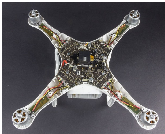
Figure 3.1 The inside of a DJI Phantom III UAV, which has plenty of connections and components to target for an adversary. Photo by Raimond Spekking, under Creative Commons 4.0 license.
