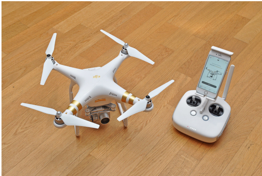
Figure 5.2 The DJI Phantom 3 Standard is a well-studied commercial UAV using a remote controller with a mobile device for control. The picture is taken by Marco Verch and is available under Creative Commons License 2.0.
