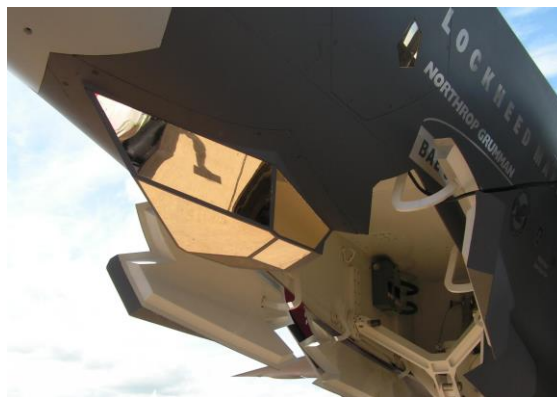
Figure 1. The segmented window protecting the EOTS system of the F-35 Lightning II. https://upload.wikimedia.org/wikipedia/commons/1/18/F-35_EOTS.jpeg
