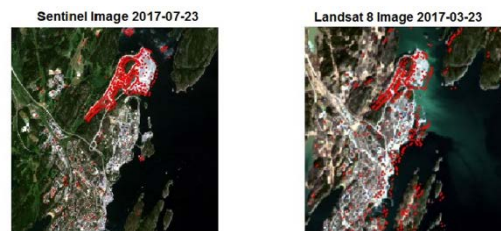
Figure 13 The detected changed pixels shown both in Sentinel-2 and Landsat-8 in approximately four months gap.
