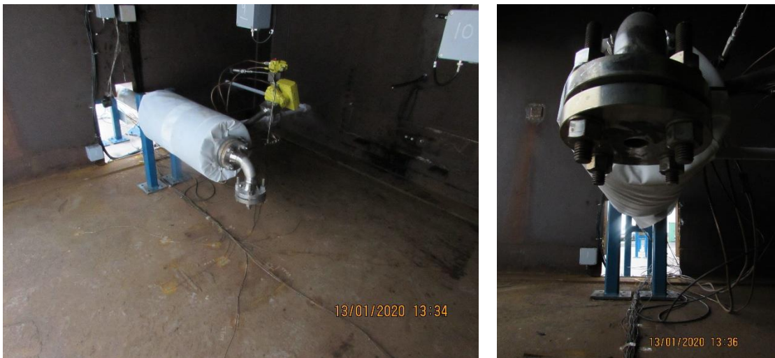
Figure 3.4 Vertical downward release orientation in closed room and ventilation mast tests.
