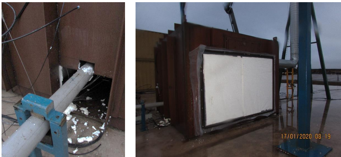
Figure 3.21 Removal of sealing around inlet of LH 2 (left photo) in Test14. Sealing of vent panel with a double layer of polyethylene with a polystyrene sheet between to the right.
