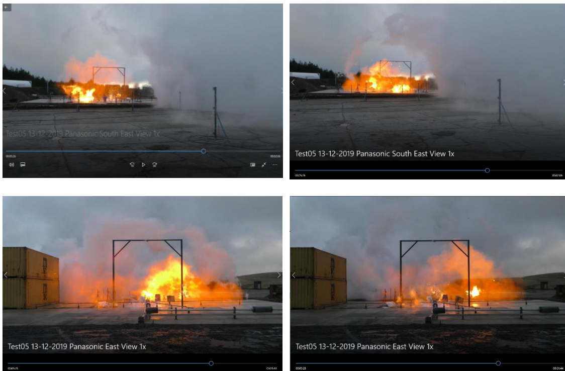
Figure 2.11 Photos from Test 5 taken during the jet fire resulting from ignition of the LH 2 release.
