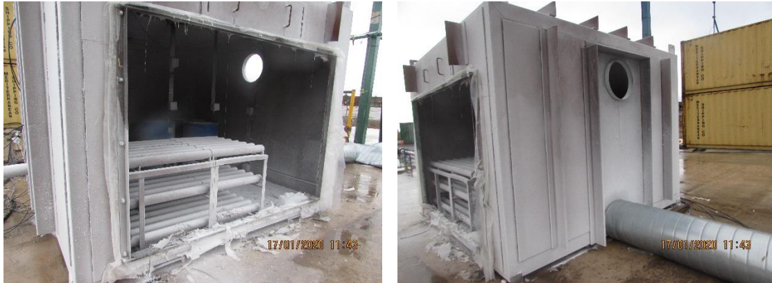
Figure 3.23 TCS after completion of Test 15. The vent mast on the photo to the right is lying on the ground after it was destroyed in the prior test. The vent mast is not connected to the TCS.
