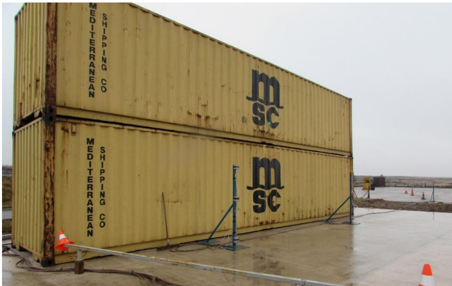
Figure 2.8 Placement of field temperature and oxygen sensors in front of the ISO container.
