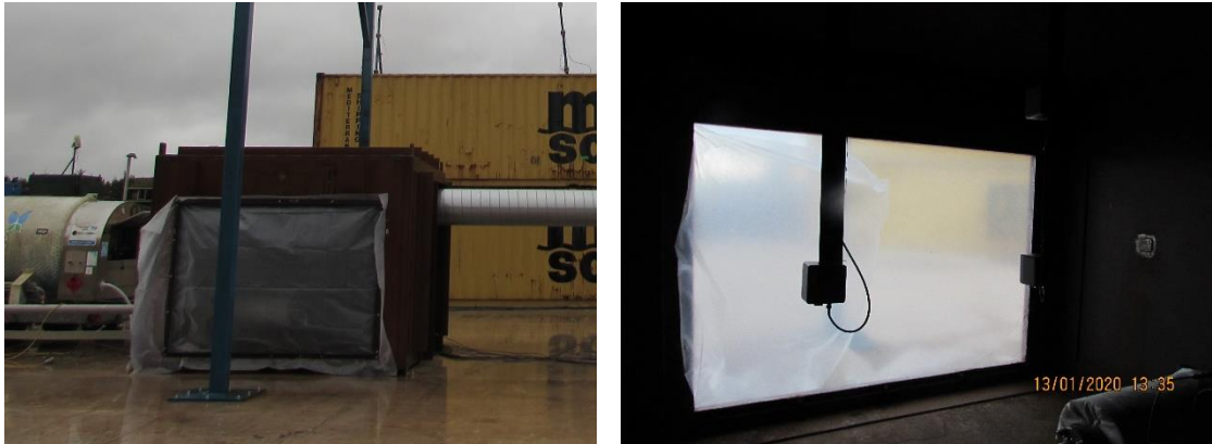
Figure 3.3 Polyethylene sheet cover seen from the outside and inside of the TCS.
