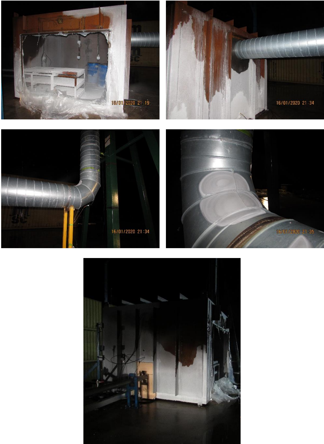
Figure 3.20 Photos of the TCS and vent mast after completion of Test 13.
