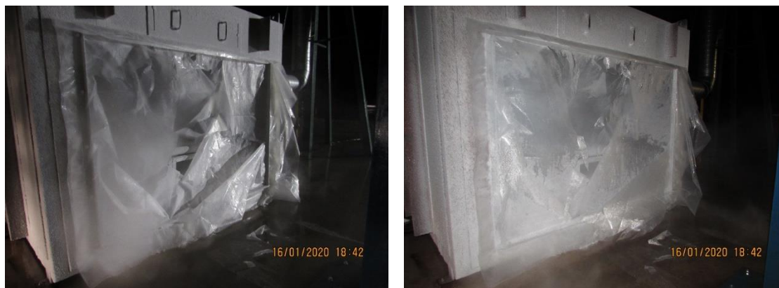
Figure 3.17 Photos of TCS after completion of Test 12. The double polyethylene sheet sheared when nitrogen was purged into the TCS saturated with \text{H}_2 .
