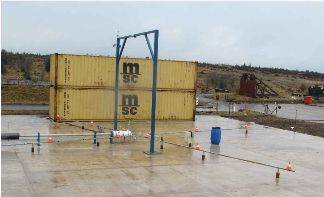
Figure 2.1 Test site with obstacles. The obstacles were two containers on top of each other, simulating a shipside, a plastic drum and an instrument box.
