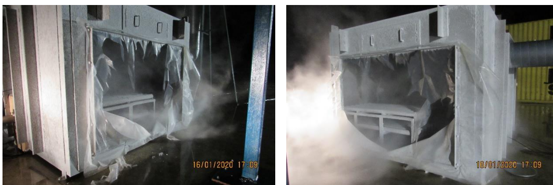
Figure 3.16 The polyethylene sheet ripped when LH 2 was released into the TCS purged with N 2 in Test 11.
