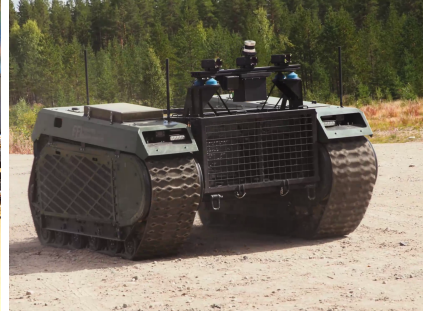
(a) CAD drawing of UGV sensor rig (b) Sensor platform with sensors in the form and sensors mounted (c) UGV Tor with sensor-rig
