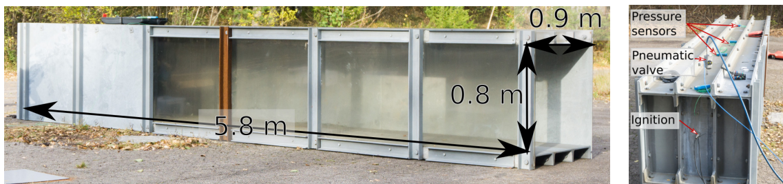
Figure 2.1 Picture of the explosion channel. The left frame shows the full geometry, whereas the right frame shows a view from the closed end of the channel.
