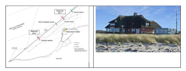
The Aschau range is located in the Eckernförde bay near the city of Eckernförde in Germany. Aschau is a multi-influence range consisting of acoustic, magnetic, electric and pressure field sensors. The range depth is approximately 21 meters. The range is secured as a military restricted area. The main objective of the range is to determine underwater signatures as function of all relevant ship parameters, like speed and diving depth with sufficient signal to noise ratio.
