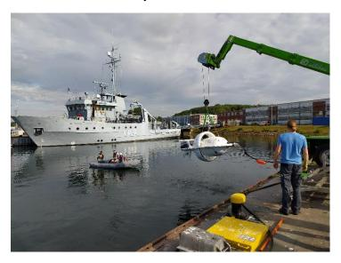
The EEG/V prototype is a new submersible version of EEG. This completely new design is more streamlined and hydrodynamically stable. It contains two coils (horizontal and vertical) to generate the static magnetic field. The module is slightly buoyant and is kept at a predefined depth using a specially designed depressor.
