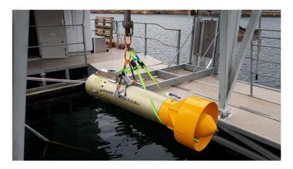
The CP-AAG (Cable Powered Advanced Acoustic Generator) is an acoustic noise source designed for sweeping acoustically activated sea mines. CP-AAG was developed by Thales Australia and is based on the operational system Advanced Acoustic Generator (AAG). The main difference is that the CP-AAG utilizes 3-phase power supply from the towing vessel in
