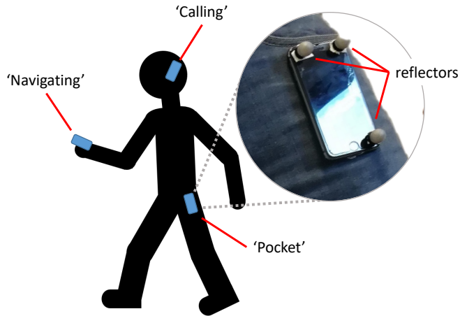
Fig. 1. The three fixed phone positions considered in this study. The 'Pocket' position is heavily influenced by short-term rotations related to the walking motion, whereas the 'Calling' and 'Navigating' positions are relatively stable. The 'Pocket' position is thus the more challenging scenario (see also Fig. 2). Rigid body tracking is based on the three reflectors in the corners of the phone.
