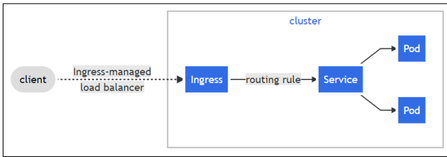
Figure 18: Example of an ingress controller process [31].
