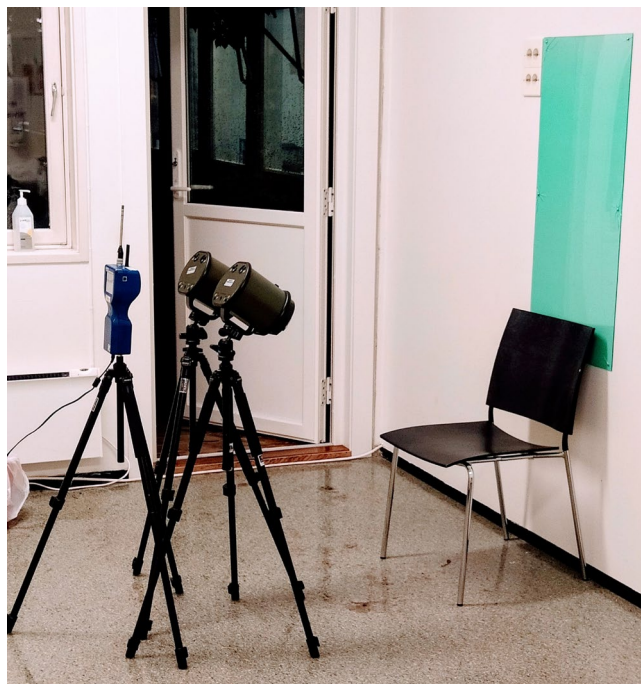
FIGURE 1 Setup used in preliminary testing, with two SASS3100 air samplers in parallel and an Aerotrak 8220 optical particle counter
