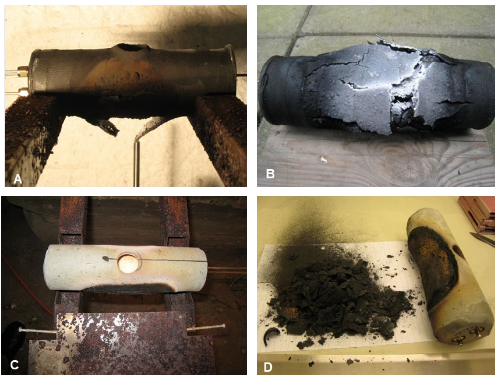
Figure 5 A-B) Effect of heat exposure on the PFP materials, exemplified by Exp 2.1 (steel tube with Firestop); C-D) Effect of heat exposure on the PFP materials, exemplified by Exp 3.1 (steel tube with Jotachar);
