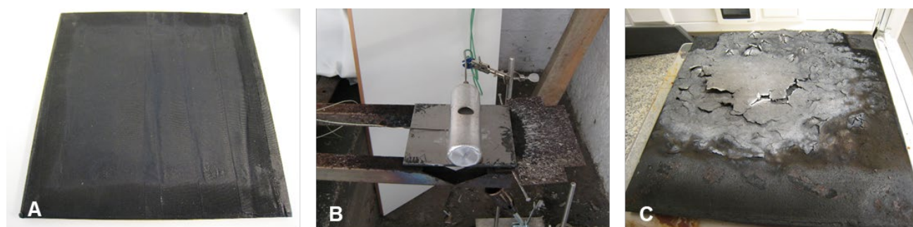
Figure 7 A) 200 x 200 mm aluminum plate (5 mm) vulcanized with 2.5 mm Firestop; B) Experimental set-up; C) Protected plate after heat exposure for more than 120 min.
