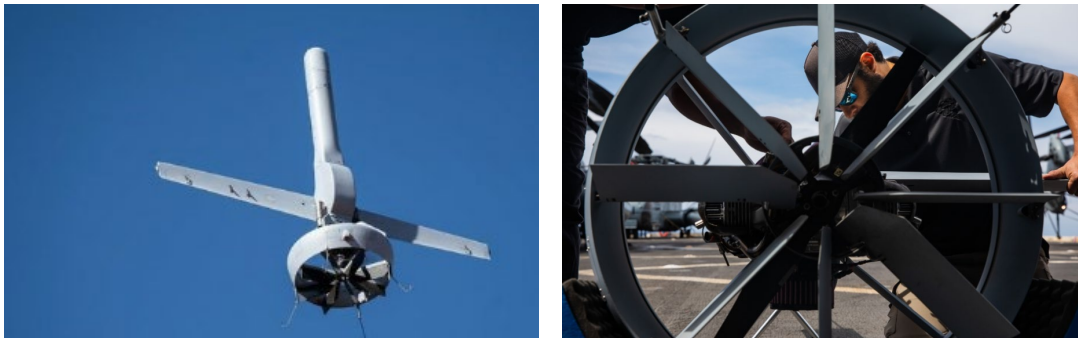
Figur 4.3 Shield AI V-BAT ( ducted fan med thrust vectoring [1] )
