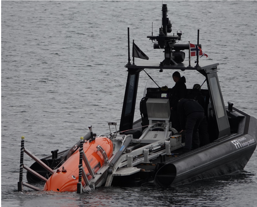
Figure 2.2 Stinger in Launch position with its carrier extended, ready to release the AUV.
