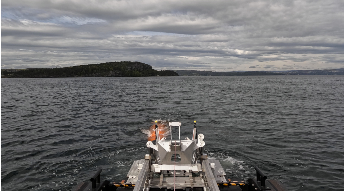
(a) End of Phase 4. Hugin's lateral alignment is clearly too far off center.
