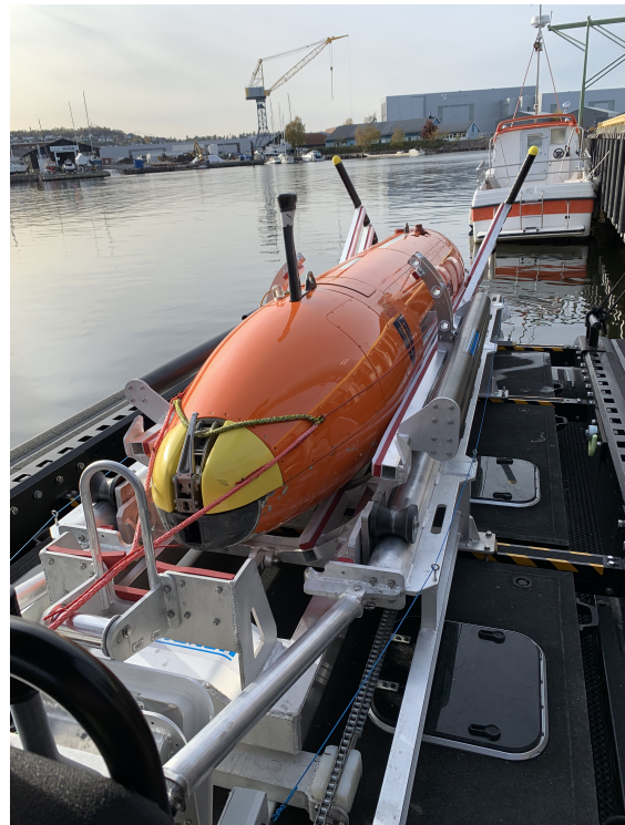
(a) Winch line (yellow rear part) will catch the nose hook (b) Winch line (yellow part) caught in the nose hook during recovery.
