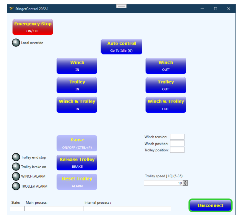
(b) Direct manual control of winch line and trolley.
