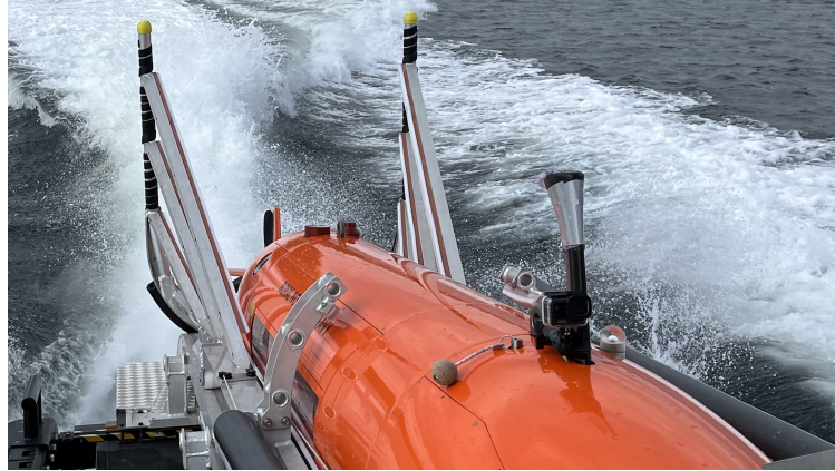
Figure 4.1 Retroreflective tape attached to the antenna for simplified detection with lidar.
