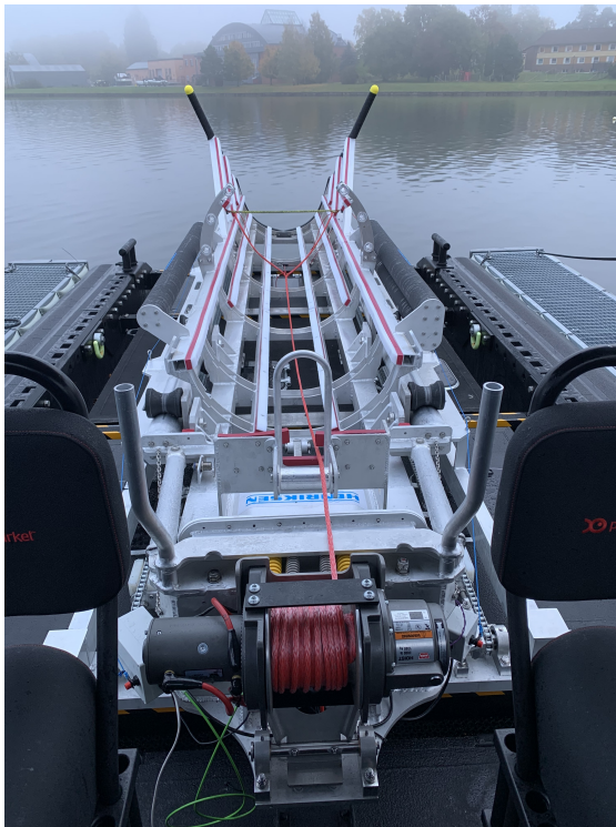
(a) Winch line (yellow rear part) will catch the nose hook (b) Winch line (yellow part) caught in the nose hook during recovery.
