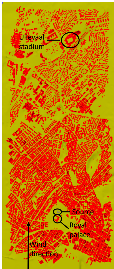
Figure 3.1 The geometrical domain for the full-scale urban simulations. The source location is indicated just north of the royal palace. The average wind direction from the south is indicated with the arrow.
