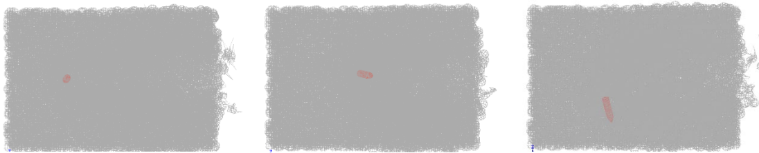
Figure 6.3 Final state with impact point skewed from central impact. Left: (x,y) = (-10,0) cm, Middle: (x,y) = (0,10) cm, Right: (x,y) = (0, -10) cm. ( x -axis is into the plane).
