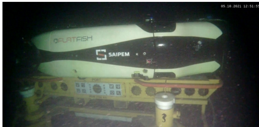
Figure 15. Vehicle successfully landed on the docking plate.
