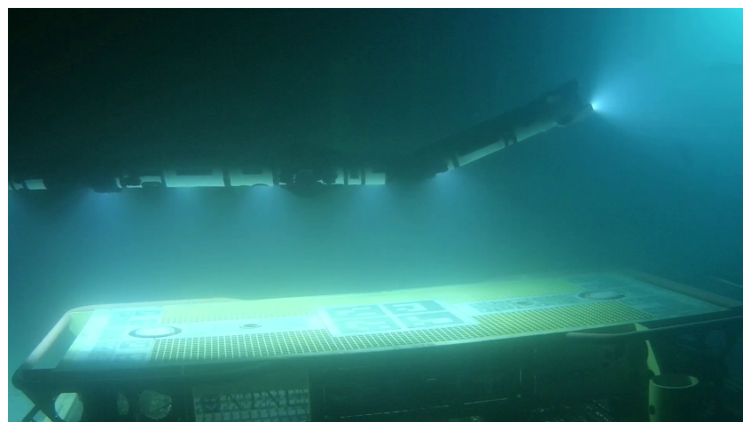
Figure 6. Eelume vehicle close to the docking station. Image taken by the camera at the subsea site (observation rig).
