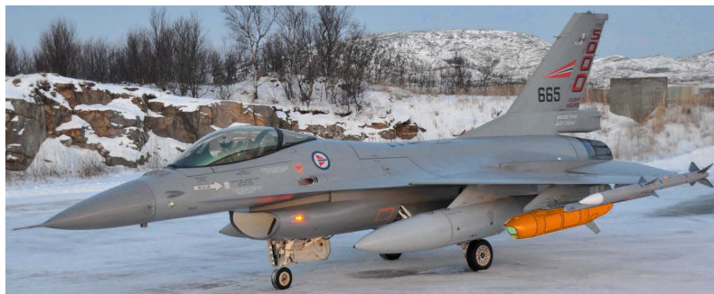
Figure 1. A research pod (illustrated in orange) will be mounted on an F-16 aircraft wing for data acquisition and ATR algorithm tests at high speeds.
