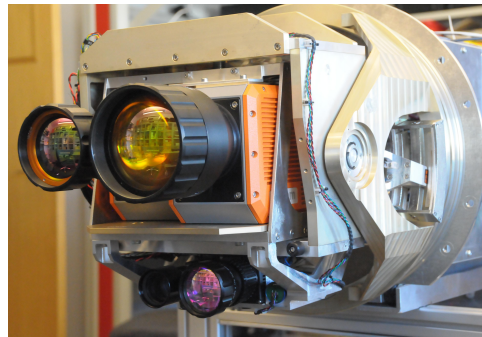
Figure 3. The camera platform located in the front of the pod is steerable in the yaw and pitch directions. Four cameras are mounted on the platform; the orange LWIR and MWIR cameras on the top, and the black SWIR and visible cameras below.
