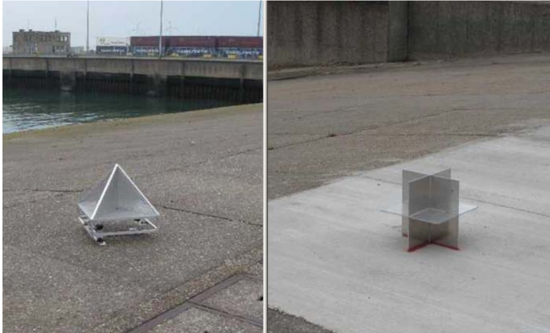
Figure 1 Two of the radar corner reflectors that were deployed in Zeebrugge harbour by Fraunhofer IOSB in (left) and Royal Military Academy (right). The size of the reflectors are around 0.5 m.
