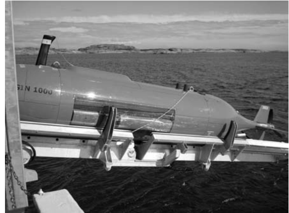
Fig. 1. The HUGIN autonomous underwater vehicle equipped with the HISAS wideband interferometric synthetic aperture sonar.
