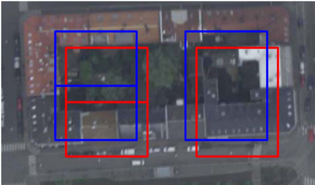
Fig. 1. (Color online) Illustration of the trade-off between coregistration error and pixel count. The figure illustrates the pixel footprint for two bands, shown as red and blue rectangles, for two cases. There is a fixed amount of spatial distortion, caused by the imaging optics or other imperfections in the imaging process. On the left is a case with small pixels and a spatial coregistration error that is a large fraction of the pixel size. On the right is a case with larger but fewer pixels. Then the relative amount of distortion is reduced, and also the signal-to-noise ratio improves. The scene is assumed to contain contrasts on a wide range of spatial scales, illustrated here by an urban landscape. Here it is not obvious how to make the important trade-off between coregistration and spatial resolution in spectral imaging. This paper proposes information capacity as a relevant figure of merit.
