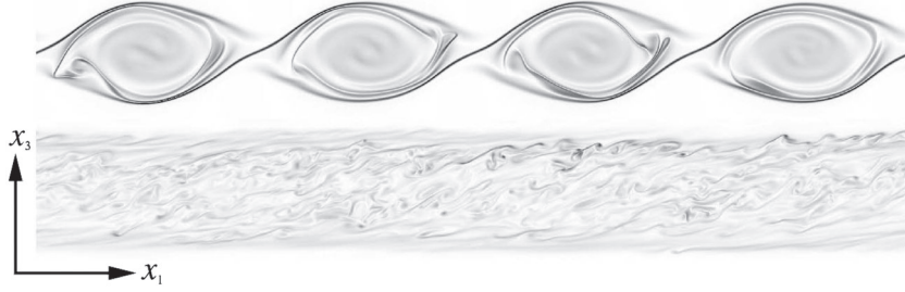
Figure 1. Contours of instantaneous vorticity magnitudes at (top) t^* = 50 and (bottom) t^* = 227 . C.f. also Figures 2 and 3.
