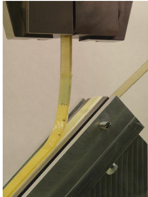
Figure 4 Fixed arm peel test at 45^\circ . (a) Before the test, and (b) detail from the initial test phase.
