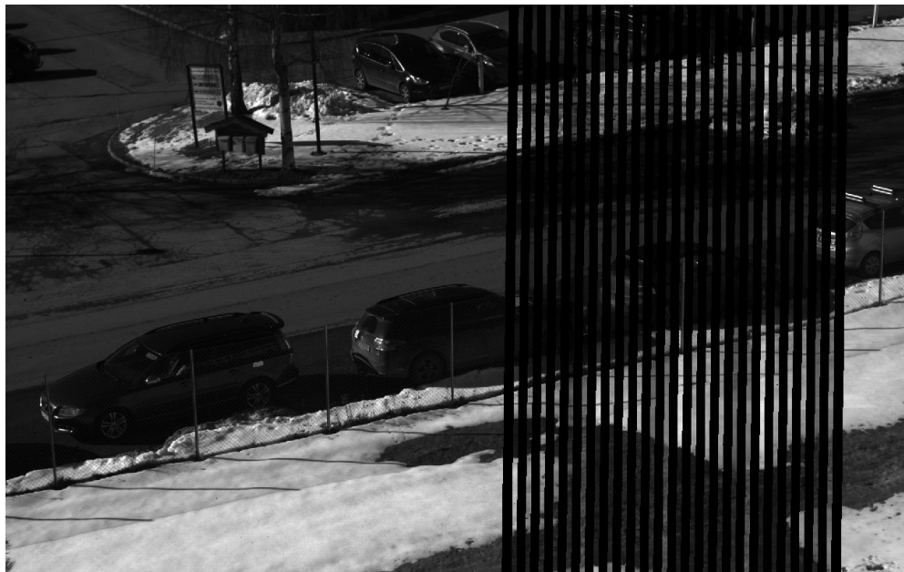
Figure 3. Raw image from a camera, with the actual filter array seen on the right. (The brightness has been adjusted in the filter region for visual clarity.)
