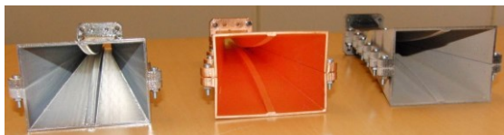
Fig. 6: WRD750 horn antennas 3D printed and metallized split in two
