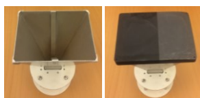
Fig. 2: Horn antenna with (right) and without 3D-printed radome (left)
