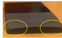
Fig. 3: Radome with unintentionally curved edges
