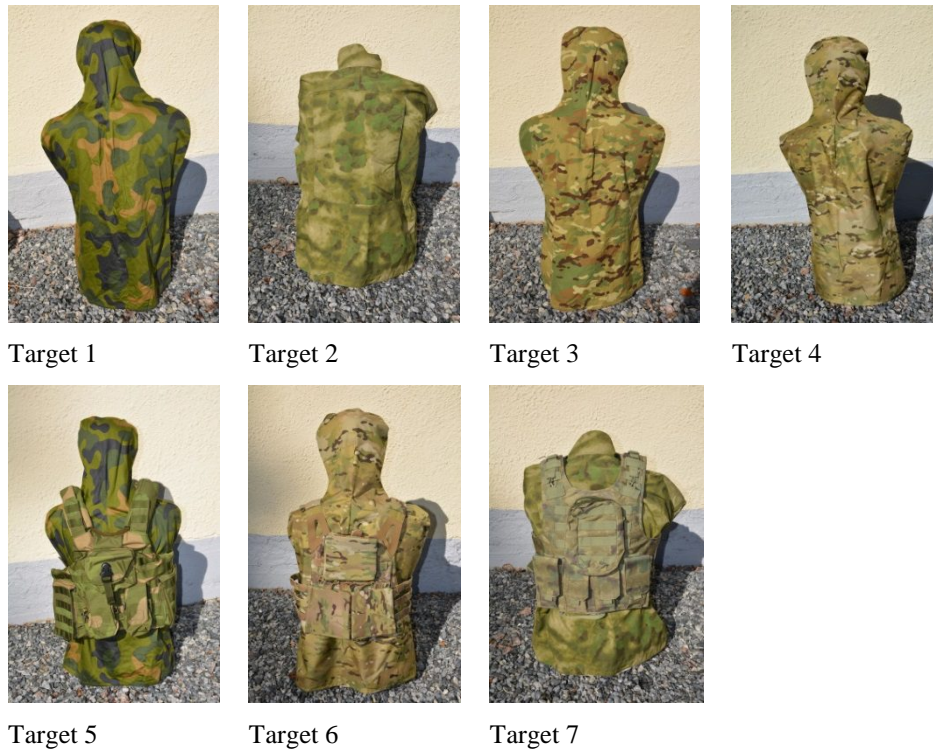
Figure 2 The camouflage patterns used in this study. We see that the study included targets dressed in suits with camouflage pattern and targets with additional vests with pouches above the suits. The vests and pouches matched the pattern of the underlying suits.
