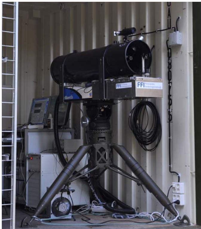
Figure 3.7 Lidar located in 10 feet instrument container
