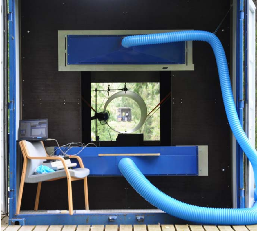
Figure 3.6 The instrument container as seen through the release container, 210 m behind. The size of the laser beam inside the test chamber is slightly smaller than the cross section of the instrument container as viewed in the picture
