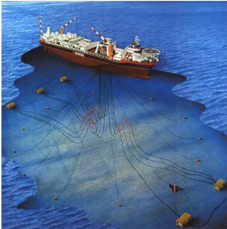
Figure 3.9 The oil production vessel, Norne FPSO, moored to the ocean bottom. © Statoil.
