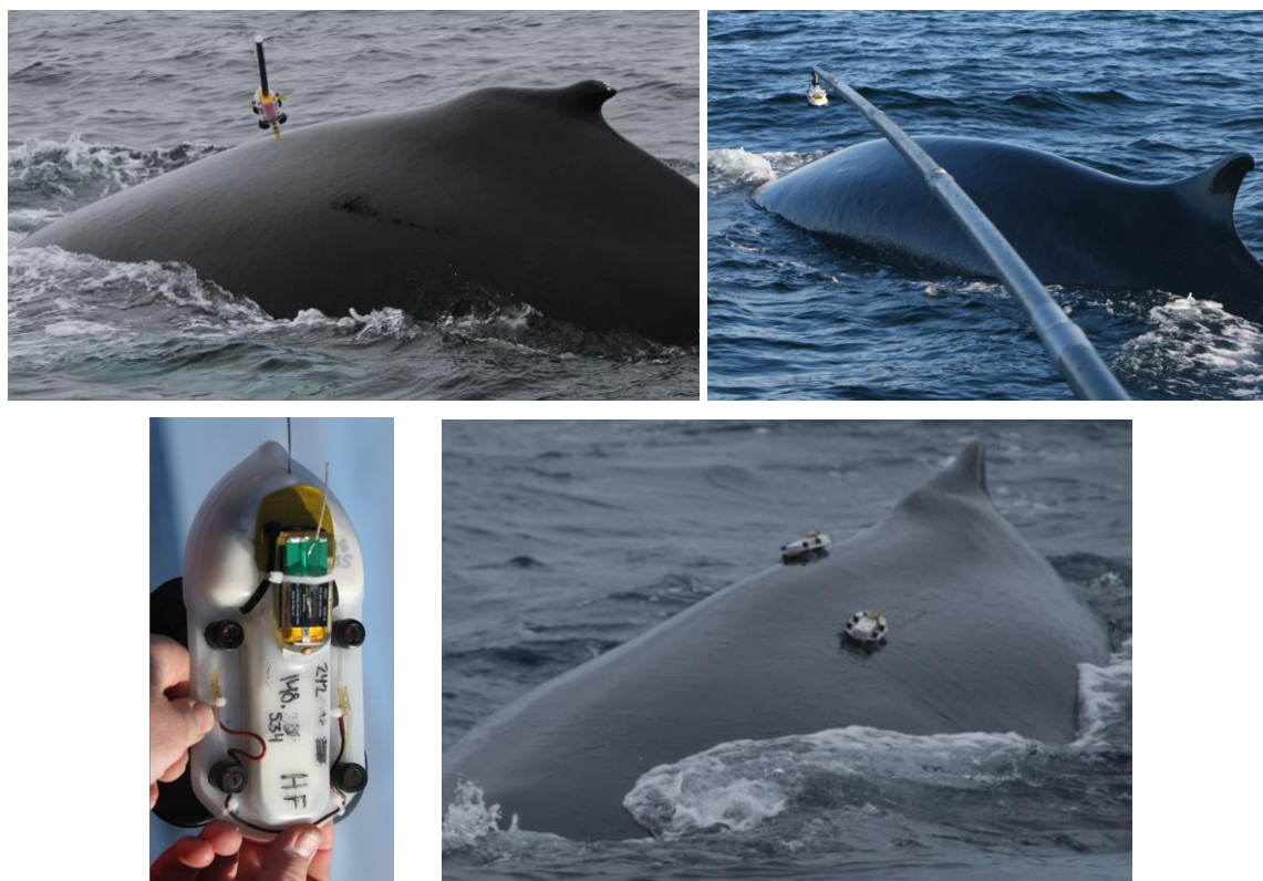
Figure 2.1 The ARTS system (upper left) and the cantilever long pole system (upper right) were used in parallel to tag humpback whales and fin whales with suction cup attached DTAGv2 tags with a Sirtrack GPS logger piggybacked to it (lower left). Animals were often double tagged to increase the chance that at least one tag stayed attached for the entire duration of the 15 hr experiment (lower right). Photo clockwise; Paul Ensor, Rune Roland Hansen, Paul Ensor, Lars Kleivane.
