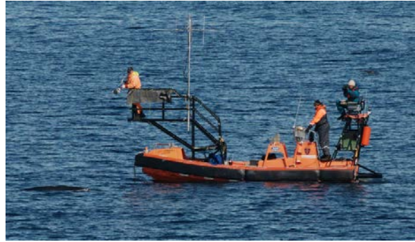
Tag boat 1 (left) and Tag boat 2 (right). Tag boat 1 will be equipped with a swivel in the bow for the cantilever pole. Tag boat 2 has a 2 person elevated MMO-station behind the driver for the tracking phase, and an elevated shooting platform in the bow for the tagging phase.
