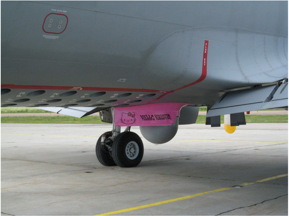
Figure 1.2 The fairing (in pink) mounted on the radome and fuselage.
