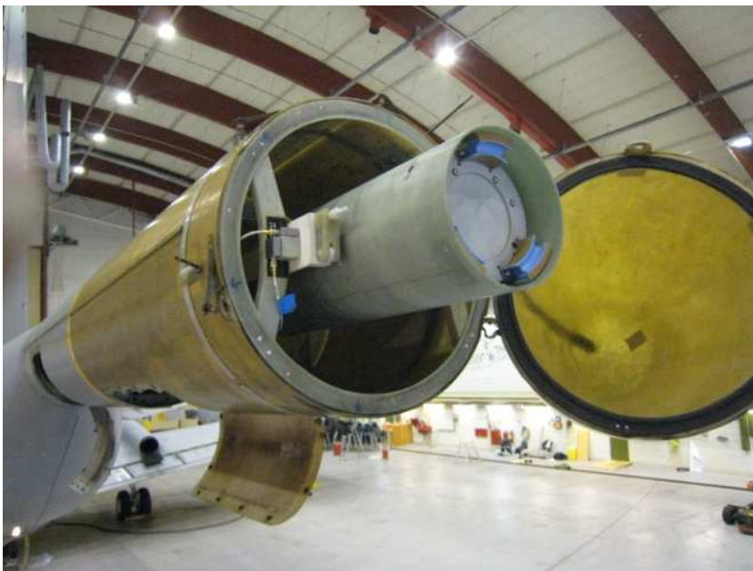
Figure 2.3 Accelerometer mounting at boom2.
