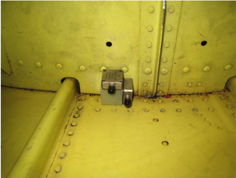
Figure 2.2 Accelerometer mounting at empennage1.
