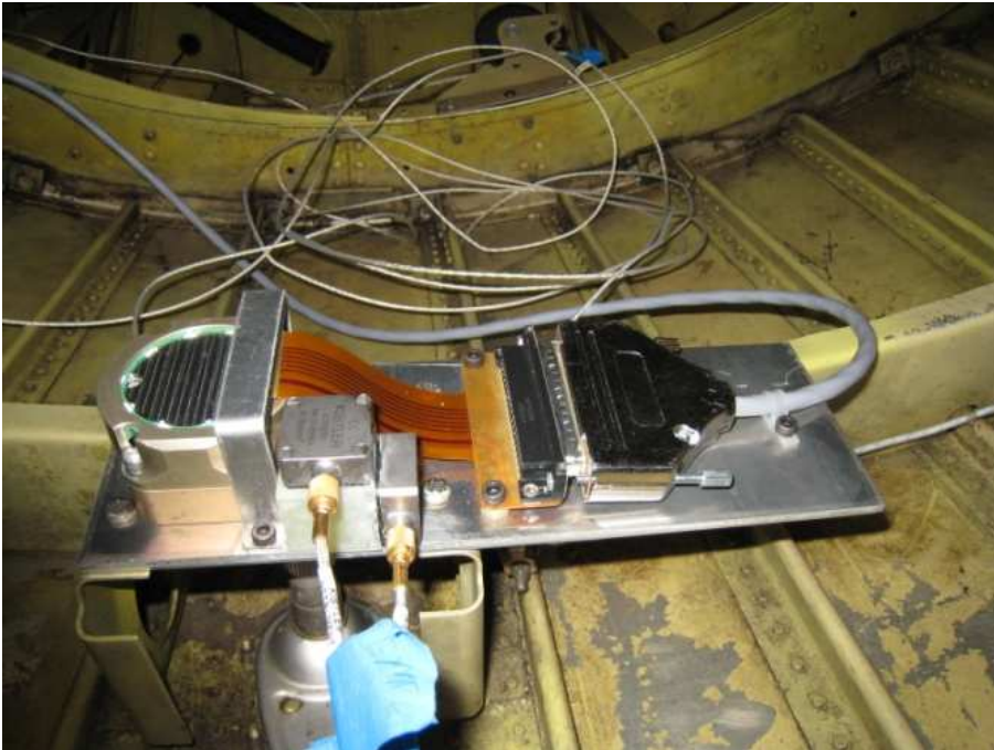
Figure 2.4 Accelerometer mounting at empennage2.
