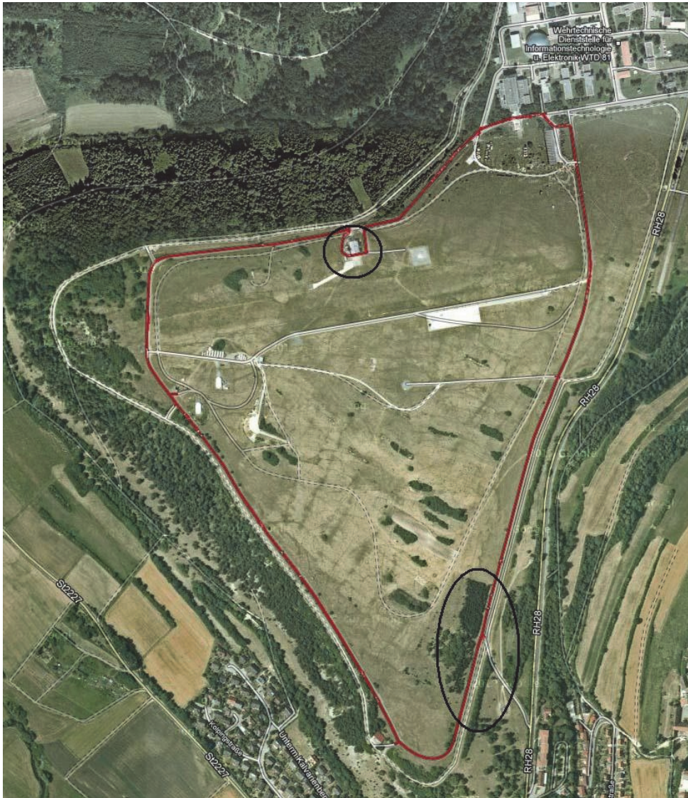
Figure 7.1 A picture from Google maps ( http://maps.google.com ) showing the field where we performed most MTR tests. The black circle at the top shows the position of the tower where the gateway node was placed (DEU5). The circle at the bottom shows an area where there were bad channel conditions on the UHF frequency band.
