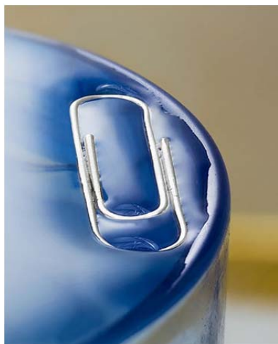
Figure 3.2 A metal paper clip is held on water surface due to its high surface tension [28]
