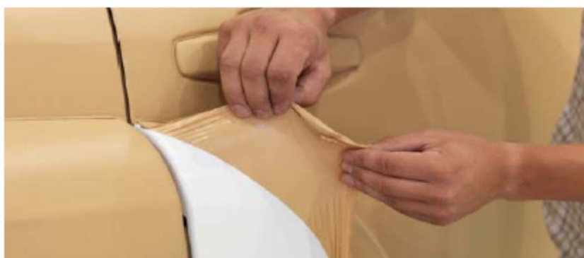
Figure 4.8 Intergard® 10220, the chemical agent absorbing coating can be easily removed from the surface [78].
